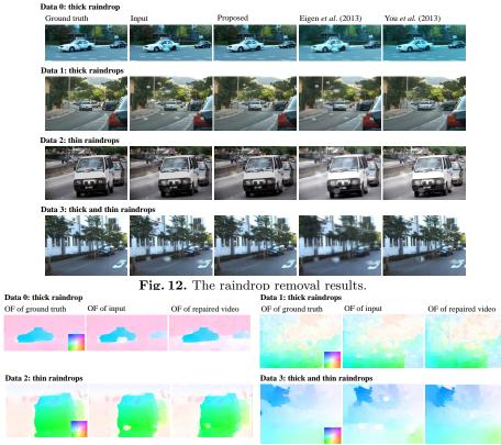
Fig. 13. Comparison on motion field estimation before and after raindrop removal. Repaired motion field Fig. 13 shows the results of the motion field estimation, before and after the raindrop removal. As shown in the figure, our method can improve the dense motion estimation, by removing the raindrops, and then repairing the motion fields.
